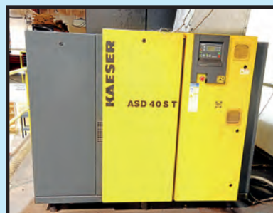
KAESER 40 HP ROTARY SCREW AIR COMPRESSOR
