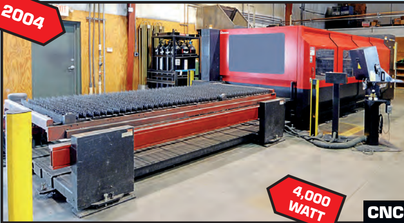
AMADA MDL. FO-3015NT CNC LASER CUTTING MACHINE
