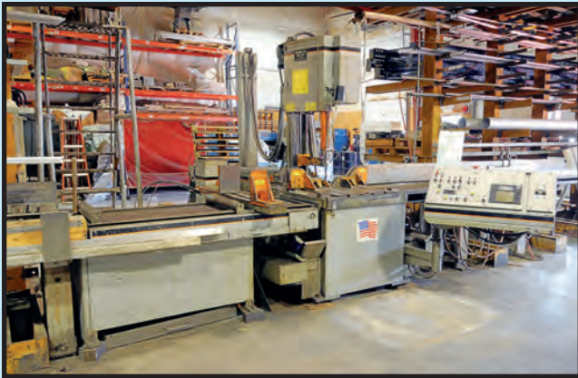
HE&M MDL. VT120HA AUTOMATIC TILT-FRAME VERTICAL BANDSAW
