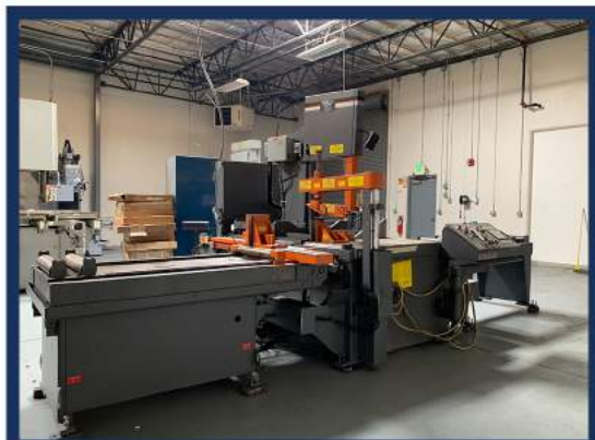
Hem Saw VT120HA-60 Vertical Cutting Production Band Saw, Capacity: 18" W x 24" H @ 90 degrees
