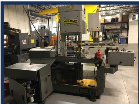
Hyd-Mech V18 Vertical Mitering Band Saw Mitering Capability: 45 degrees left to right
