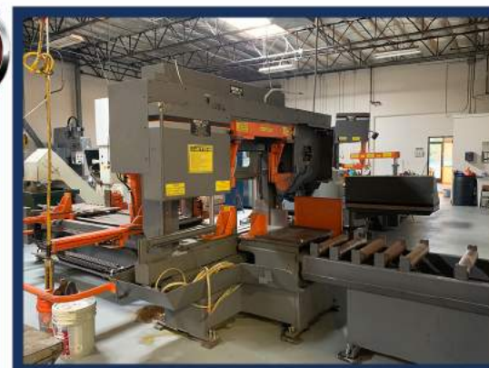
Hem Saw H130HA-DC Automatic Band Saw, Dual Column, Large 18" Round Capacity, Fully Automatic
