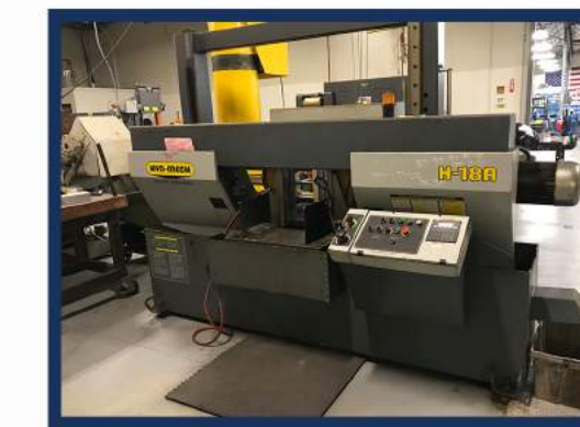
Hyd-Mech H-18A Automatic Horizontal Band Saw, 18"H X 18"W, 10 HP
