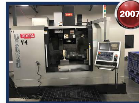
2007 Toyota BM-1200 CNC VMC, Fanuc 18i-MB Control, CAT 50 Taper, High Pressure Coolant, Chip Conveyor, 4th Axis Ready, 30 ATC
