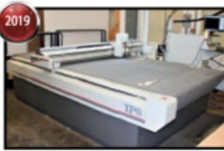
2019 TPS Mdl. S-1 Digital Laser Cutter w/Bevel Attachment
