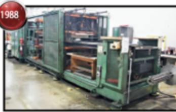
1988 Sencorp Mdl. 2500 Inline Thermoformer
