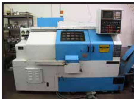
SUPERMAX YCM TC-2 CNC LATHE WITH FANUC OT CONTROL, 6" CHUCK, TAIL STOCK, 8 STATION TURRET, CHIP CONVEYOR, S/N 507321
