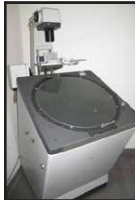
MITUTOYO PV-600 24" OPTICAL COMPARATOR, SERIES 305, S/N 9282.
