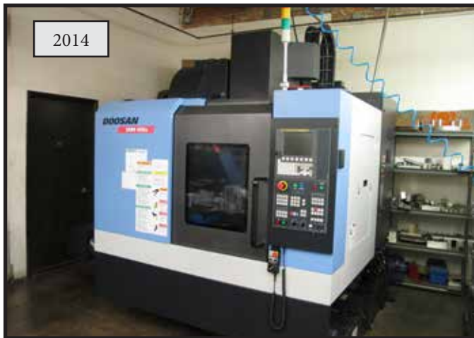
2014 DOOSAN DNM 400a CNC VMC, CT-40, 20 ATC, FANUC I CONTROL, 30" X 17.1" X 20.1" (XYZ), S/N MV0038-000283.
