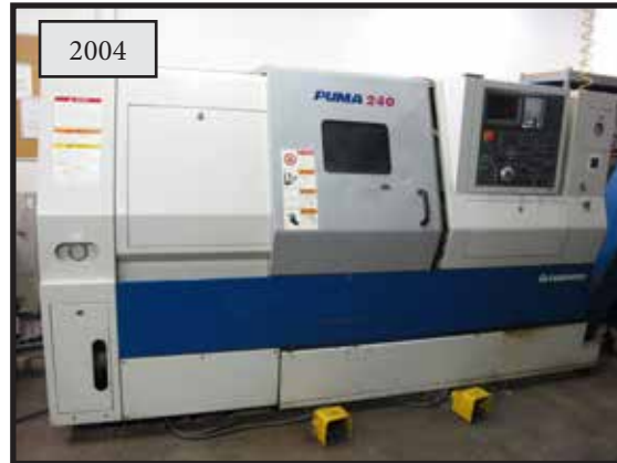
2004 DAEWOO PUMA 240 CNC LATHE, 8" CHUCK, TOOL SETTER, TAIL STOCK, 12 POSITION TURRET, CHIP CONVEYOR, S/N 240608.
