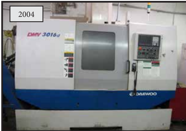
2004 DAEWOO DMV 3016D CNC VMC, CT 40, 20 ATC, 30" X 16" X 20" (XYZ), 8000 RPM
