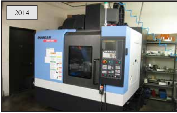
2014 DOOSAN DNM 400a CNC VMC, CT-40, 20 ATC, FANUC I CONTROL, 30" X 17.1" X 20.1" (XYZ), S/N MV0038-000283.
