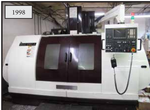
1998 CHEVALIER 2552 VMC WITH FANUC O-MD CONTROL, 20 ATC, CT-40, 52" X 25" X 25" (XYZ).
