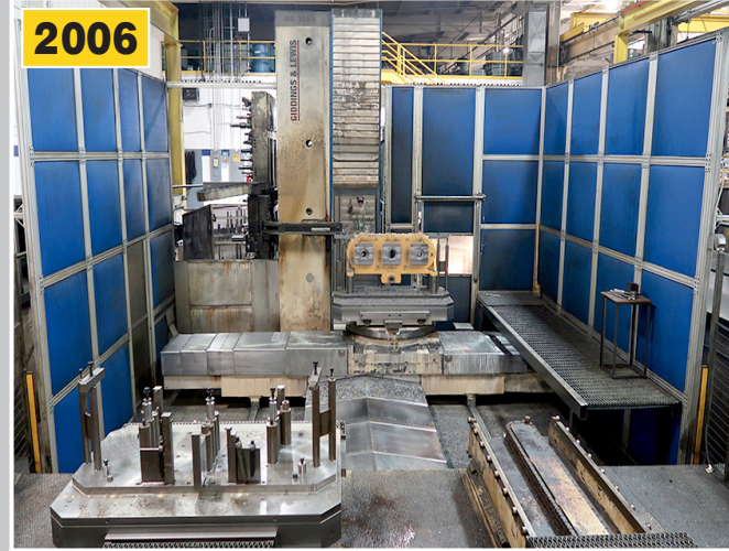
GIDDINGS & LEWIS MC 1250 6.1" CNC Horizontal Boring Mill
