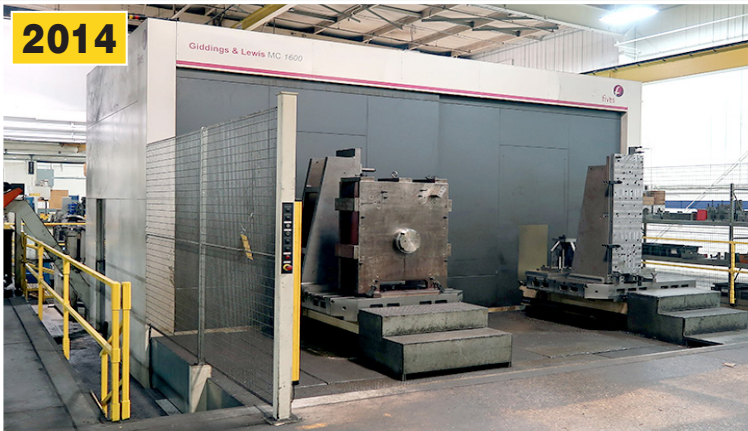
2014 FIVES GIDDINGS & LEWIS MC 1600 6.1" CNC Horizontal Boring Mill
