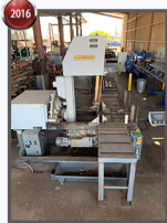
2016 Hydmech V-20, 60 degree mitre, 25" x 20" Rectangular capacity, 20" round capacity
