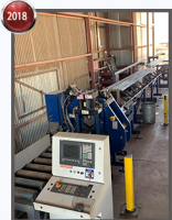
2018 Peddinghaus Ocean Clipper Angle Line, Drill 13.5 HP, Punch 75 tons, Shear 100 tons, Angles 1.5" x 1.5" x 1/8" - 6" x 6" x 5/8"
