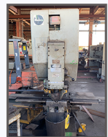
Mubea Ironworker, 120 ton, Flat/Round/Angle Shear, Punch, Notcher
