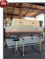
2000 Accurpress 725012, 250 ton x 12' capacity, ETS 200 Control, 2 axis backgauge
