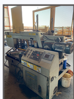
Hydmech M-20A, Automatic Horizontal Bandsaw, 20" x 30" capacity, 10HP, Mitres from 90deg to 60 deg
