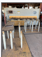
Atlantic Shear, 10' x 1/2" capacity, Powered Backgauge
