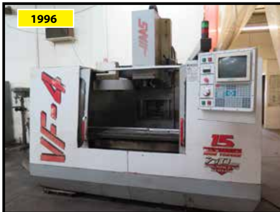
1996 1996 Haas VF-4 4-Axis CNC Vertical Machining Center s/n 8017 w/ Haas Controls, 20-Station ATC, CAT-40 Taper Spindle, 7500 RPM, Thru Spindle Coolant, 15Hp High Torque Motor, Rigid Tapping, Programmable Coolant Nozzle, Floppy Disc, 18" x 52" Table, Coolant
