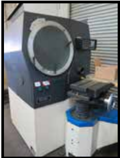
Jones & Lamson 20" Optical Comparator s/n C-509009 w/ J & L Decimetric II DRO
