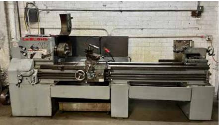
LEBLOND ENGINE LATHE, 18" X 72" CC, 10" CHUCK, TAILSTOCK
