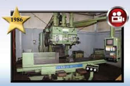
1986 OKK MH-600, Travels 51" x 21" x 23", 3 Spindle Machine with 2500 RPM, NMTB 50 Taper, Milcon V Control
