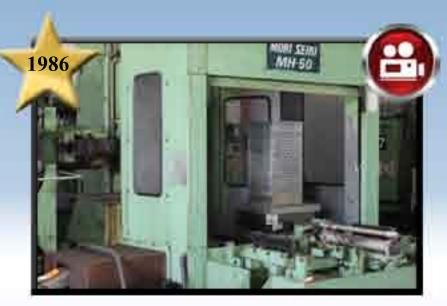
1986 Mori Seiki MH-50, 2 Pallets 19.69" x 19.69", Travel 31" x 25" x 29", 40 ATC, 4500 RPM, CAT 40, Fanuc 11M, 1 Deg
