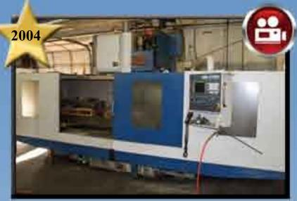
2004 KAFO MCMC 21100, Travels 84" x 39" x 39" 30 ATC, 5000 RPM, Cat50, Fanuc Control, 20 HP
