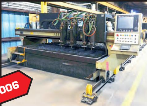
ALLTRA 4-HEAD CNC OXY. FUEL SHAPE CUTTING MACHINE
