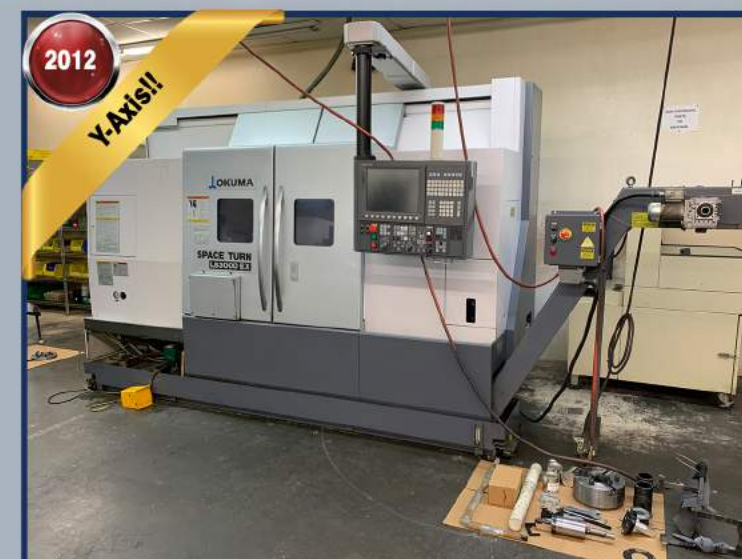
2012 Okuma LB-3000 EX-MY , SN 165078, 3.1" Bore, 2.75" Bar Capacity, Tool Setter, Collet Chuck, High Pressure Coolant, 12 Station Turret, Y Axis, Live Tooling, Tailstock, Okuma OSP-P200LA Control, Includes Tooling in Picture and 10" 3 Jaw Chuck and Accessories, 2013 Chip Blaster J30 SN- J267 1000 PSI
