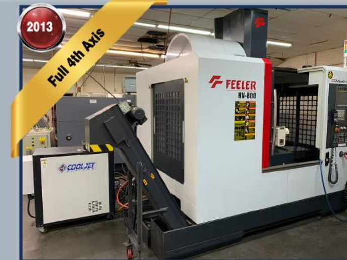
2013 Feeler HV-800 SN: HVG049 , Table Size 37" x 20", X- Axis 32", Y-Axis 20", Z-Axis 20", 15000 RPM, 4th Axis Rotary Table with Tailstock and Fixture , Tool Setter, 30 Tool Side Mount, Chip Conveyor, Fanuc Series Oi-MD Control, Remote Jog Handle, TSC, 2015 Cool Jet High Pressure Coolant System.
