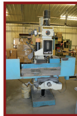
(2) 1997 Supermax YCM-40, 28" x 15.5" x 16" Travels, 4,200 RPM, Supermax CNC 400 Control, Full 3 axis Programmable
