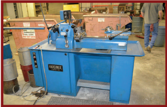
Hardinge DV59, 6 Station Turret, Footstock, with Hydraulic Barfeed 10ft.
