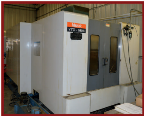
(2) 2001 Mazak VTC 160A w/2 pallets, 22" x 16" x 22" Travels, 10,000 RPM, Mazatrol 640M Control, Cat 40, 30 ATC, Chip Auger & Conveyor
