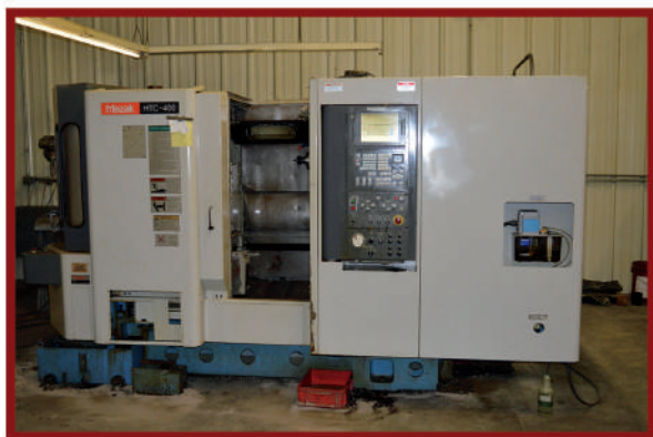
1999 Mazak HTC400, 22 x 20 x 20, Cat 40, Mazatrol 640M Controls, 30 ATC, Chip Auger, With Pictured Transformer, EIA/ISO, (2) Tombstones included
