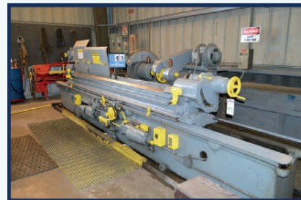
Norton Hydraulic Mechanical Cylindrical Grinder, 2" Grinding Wheel
