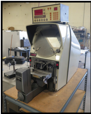
Gage Master Series 20 13" Optical Comparator w/ Gage Master GM4 DRO
