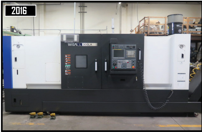
2016 Hyundai WIA L300LA CNC Turning Center w/ Hyundai WIA Fanuc i-Series Controls, Tool Presetter, 12-Station Turret, 3600 RPM, Hydraulic Tailstock, Chip Conveyor
