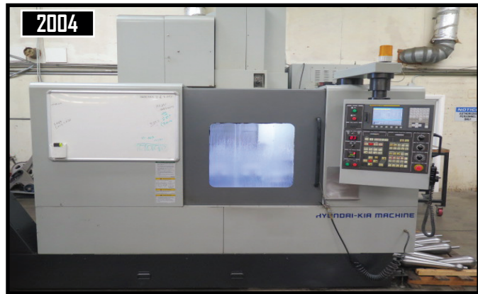
2004 Hyundai WIA VX500 4-Axis CNC Vertical Machining Center w/ Hyundai WIA Fanuc i-Series Controls, 24-Station Side Mounted ATC, CAT-40 Spindle
