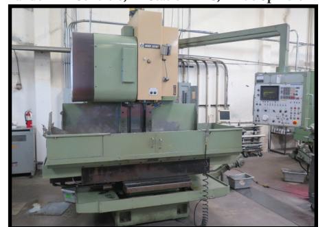
Mori Seiki MV-45/40 CNC Vertical Machining Center w/ Fanuc 6M Controls, 20-Station ATC, BT-40 Spindle
