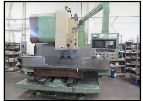
Mori Seiki MV-55 CNC Vertical Machining Center w/ Fanuc 11M Controls, 24-Station ATC, BT-50 Spindle
