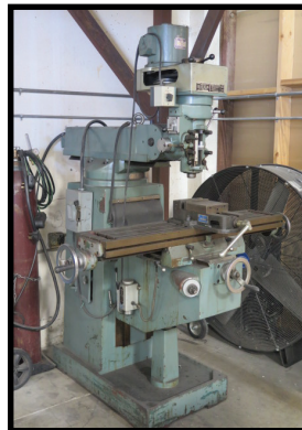
Import Vertical Mill w/ 3Hp Motor, 80-2720 RPM, 8-Speeds, R8
