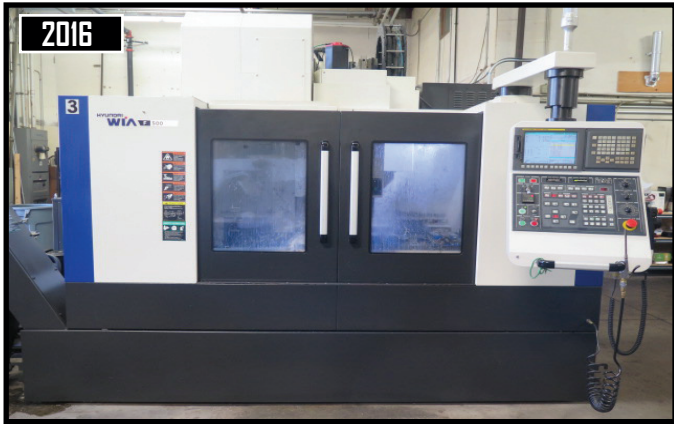
2016 Hyundai WIA F500 CNC Vertical Machining Center w/ Hyundai WIA Fanuc i-Series Controls, 24-Station Side Mounted ATC, CAT-40 Spindle, 10,000 RPM
