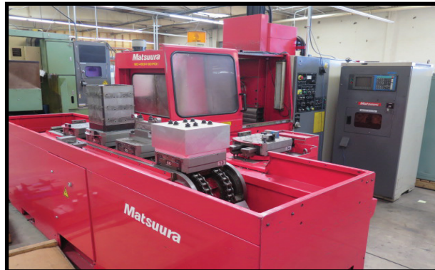
1992 Matsuura MC-450H-30-PC II 10-Pallet CNC Horizontal Machining Center w/ Matsuura Yasnac i80 Controls, 100-Station ATC, BT-40 Spindle, 10-Pallet Carousel System
