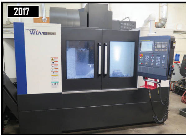
2017 Hyundai WIA KF5600 CNC Vertical Machining Center w/ Hyundai WIA Fanuc i-Series Controls, 30-Station Side Mounted ATC, CAT-40 Spindle, 12,000 RPM
