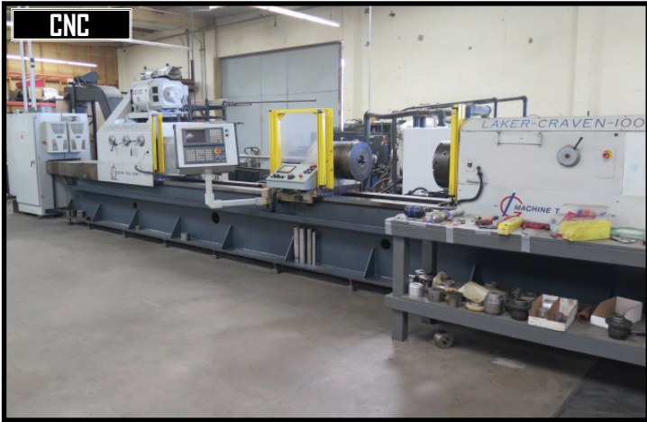
Laker-Craven-100 CNC Deep Hole Drilling Machine w/ Fanuc Power MATE Controls, 113-1818 Headstock RPM, 1760 Work-Head Spindle Speed, 110" Drilling Stroke, 20" Max Boring Diameter
