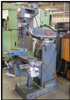
Lagun FT-1 Vertical Mill w/ Mitutoyo DRO, 55-2940 RPM, 8-Speeds, Power Feed
