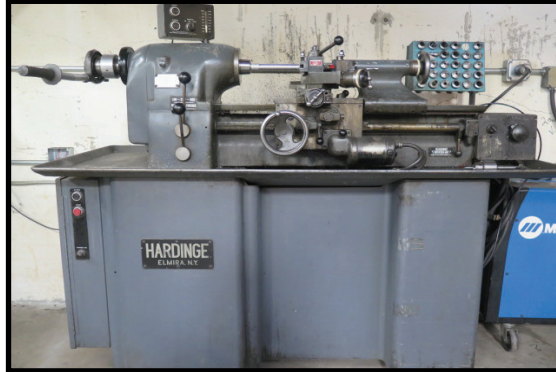
Hardinge TFB-H Wide Bed Lathe w/ 125-3000 RPM, Tailstock, Power Feed, 5C
