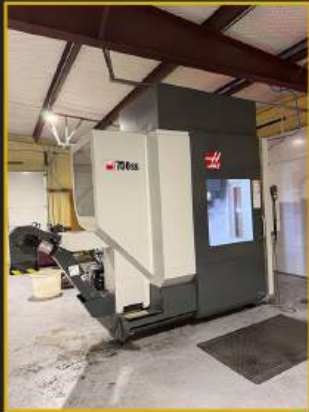
2019 Haas UMC 750SS 5-Axis Vertical Machining Center
