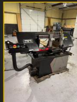
Jet Elite Horizontal Band Saw Model EHB-1018V
