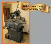
Harig Steptool Grinder Model 2023GWHAR, includes Harig Air-Flo tool box for sharpening and relieving cutters
