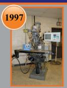
1997 Bridgeport EZ Trak DX CNC Knee Mill, Travels 30" x 12" x 16"
