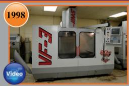
1998 Haas VF-3, Travels 40" x 20" x 25", 2 Speed Gear Box, 7,500 RPM, Auger, 4th Axis Pre Wire S/N 14279
