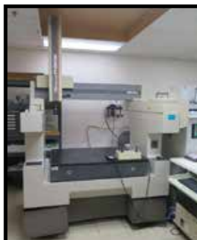
Mitutoyo FN905 CMM Machine w/ Renishaw PH9 Probe and Drive Controller, Joystick Axial Controller, miCAT MCOSMOS 3.5.4 R2 Software
