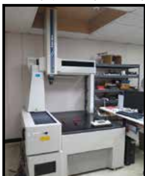
Mitutoyo Bright-A707 "Bright APEX" CMM Machine w/ Renishaw PH9 Probe and Drive Controller, Joystick Axial Controller, miCAT MCOSMOS 3.5.4 R2 Software
