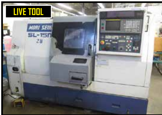
Mori Seiki SL-15MC Live Turret CNC Turning Center w/ Fanuc MF-T6 Controls, Tool Presetter, 12-Station Turret with 6-Live Stations, 5000 Spindle RPM, 2000 Rotary Tool RPM
