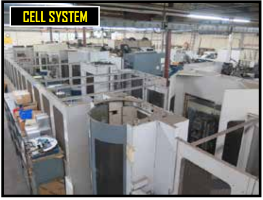
Mori Seiki Pallet Cell w/ 2000 Mori Seiki SH-503/40 Multi-Pallet HMC, (2) Mori Seiki SH-50 Multi-Pallet HMC's, 18-Station Linear Pallet Pool, Fanuc PowerMate Machine Interface System
