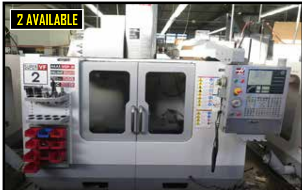
2007 Haas VF-2SSYT 4-Axis CNC VMC w/24-Side Mount ATC, BT-40, 12,000 RPM, Renishaw Wireless Probing System
