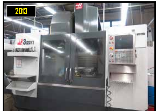
2013 Haas VF-3SSYT CNC VMC w/ 40-Station Side Mount ATC, BT-40, 12,000 RPM, Renishaw Probing System, Rigid Tapping
