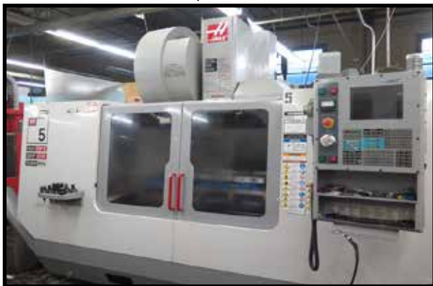
2004 Haas VF-5D/40 4-Axis CNC VMC w/ 40-Station Side Mount ATC, BT-40, 10,000 RPM, Renishaw Probing System, Rigid Tapping
