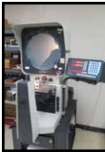
Deltronic DH214-MP-C5E 14" Optical Comparator w/ MPC-5 Programmable DRO, Digital Angular Readout, Shadow Detector
