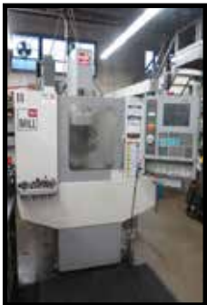
2006 Haas "Mini Mill" 4-Axis CNC VMC w/ 10-Station ATC, BT-40, 6000 RPM
