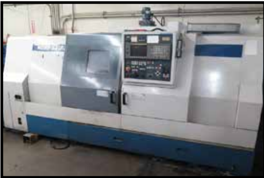
1996 Mori Seiki SL-150S Twin Spindle CNC Turning Center w/ MSC-518 Controls, Tool Presetter, 12-Station Turret, 5000 RPM on Main and Sub-Spindles
