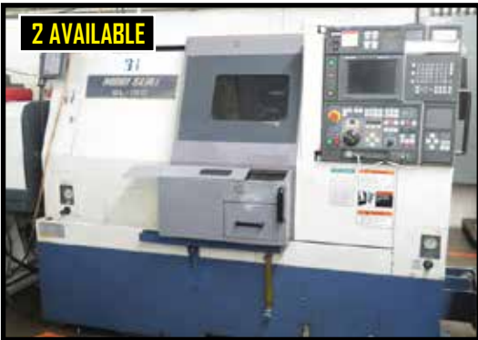
1999 Mori Seiki SL-150SMC Twin Spindle - Live Turret CNC Turning Center w/ MSC-501 Controls, Tool Presetter, 12-Station Live Turret, 40-5000 Main and Sub Spindle RPM's, 3000 Rotary Tool RPM
