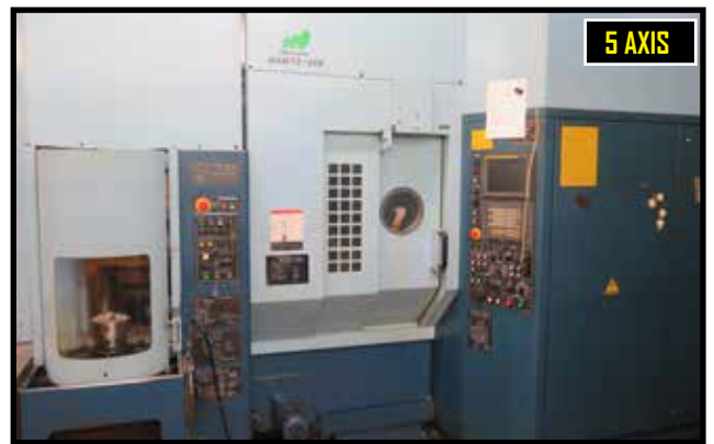
2001 Matsuura MAM-72-3VS 5-Axis Multi Pallet CNC VMC w/ Fanuc 16i-M Controls, 40-Station Tower Pallet Chuck System, 240-ATC, BT-40, 15,000 RPM, True 5-Axis Trunnion System, Renishaw Probing System
