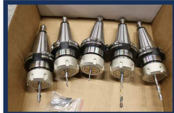
(5) CAT 40, High Speed, Balanced 20K RPM Max G2.5 (Glacern) ER-32 Collet Holders
