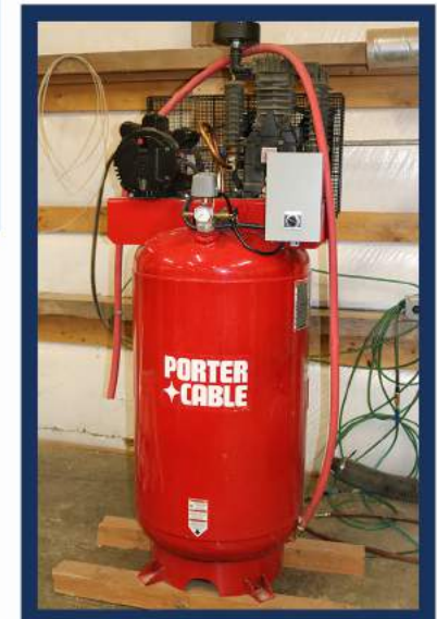
Porter Cable 80 Gallon Air Compressor, 7.5 HP, 175 PSI Max Pressure, Displacement 29.5 CFM, 1330 RPM, Model CPLMC-7580V2C
