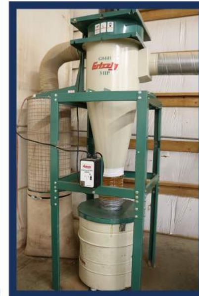
(2) Grizzly G0441, 3 HP Cyclone Dust Collector, 55 Gallon Drum, 8" Intake Hole, Impeller Size 15-1/2" Steel, Riveted, 1654 CFM at 2.0" SP
