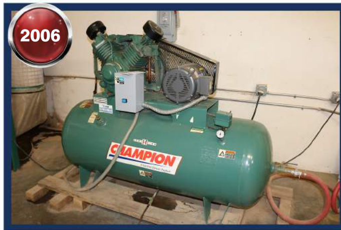
2006 Champion Centurion II 120 Gallon, 2 Stage Air Compressor, 200 Max PSI, 15 HP, Model CCSRVA, Reed Valve 5
