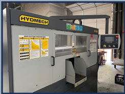
Hyd-Mech H-14A, Rectangular Capacity at 90° 14" H x 14" W, Blade Size 1 1/4" x 15' 2", Blade Drive 8.8 HP Operation Automatic
