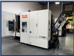
2013 Mazak HCN 4000-III, Pallet Size 15.75" x 15.75", CAT40 18,000 RPM Spindle with 47HP, Mazatrol Matrix Nexus 2 Control, 80 Tool ATC, Coolant Thru Spindle, Renishaw OMP 60 Optical Probe, ConSep 2000 Chip Conveyor
