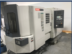
1999 Mazak HTC-400, 15.7" x 15.7' Pallet Size, 22" x 20" x 20" Travels, 40 Taper, 10,000 RPM, 15 HP, 24 ATC
