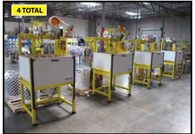
(4) 2009 HERZOG TYPE NG-1/16-140 ROUND BRAIDING MACHINES W/16 CARRIERS TENSIONER, BOBBIN 78X280 mm=1211ccm.
