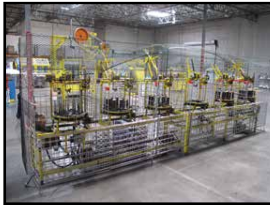
(6) BRAIDING MACHINES W/16 CARRIERS AND IN LINE ENCLOSURE
