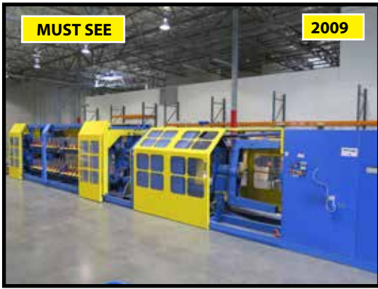
2009 MAHESH MODEL MTP20-4128 ELECTRONIC ROPE MAKING MACHINE, 128 BOBBINS SPOOLS, DIG COUNTER, COIL WINDER, AND CHEESE WINDER
