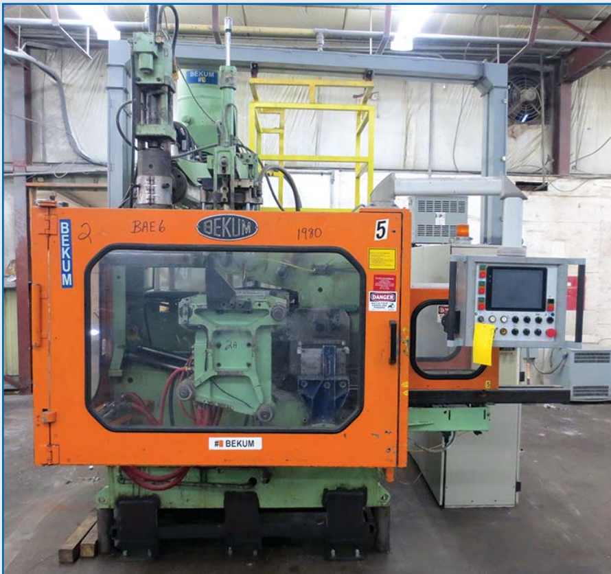
1980 (Complete rebuild in 2003) BEKUM BAE 6 single extrusion, single die blow molder with BEKUM S601 extruder, 60hp, vacuum loader, 600 volt comes with 10L 63 mm neck with handle mold s/n 52440034 #5
