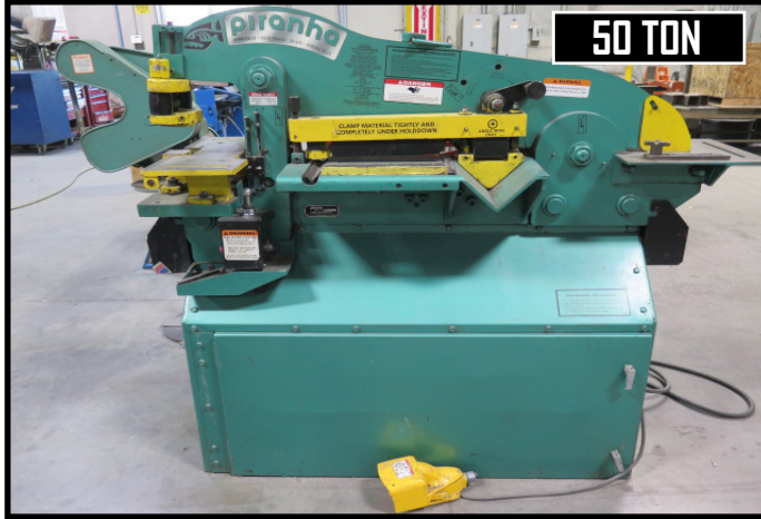
Piranah P-50 50-Ton Iron Worker
