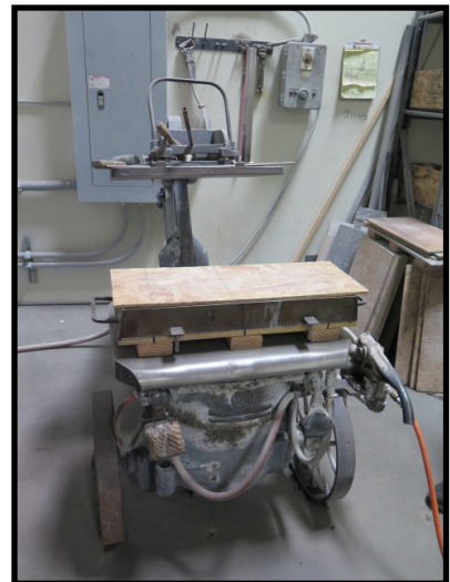
SPO Pneumatic Sand Compactor
