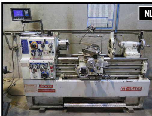
Ganesh GT-1640S 16" x 40" Geared Head Gap Bed Lathe s/n S9704-016 w/ Newall DP900 Programmable DRO, 30-2000 RPM, Inch/mm Threading
