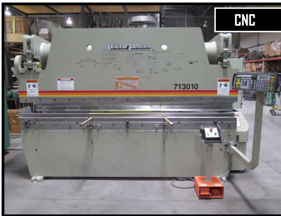
2014 Accurpress 713010 130 Ton x 10' CNC Press Brake w/ Accurpress ETS Controls, Pendant Controller
