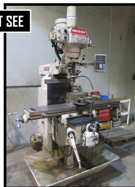
Ganesh Deluxe GMV-3 Vertical Mill s/n SV4000016 w/ Newall C80 3-Axis Programmable DRO, 3Hp Motor, 60-4200 Dial Change RPM, Power Draw-Bar
