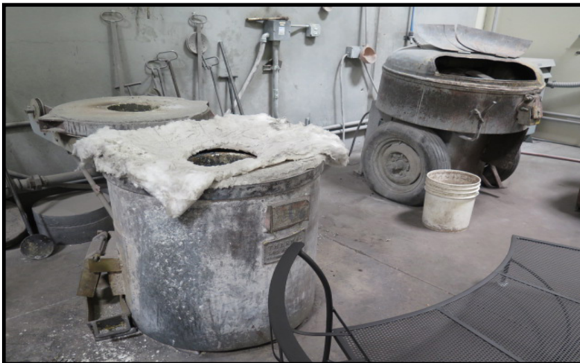
Thermal Gas Fired Furnace
