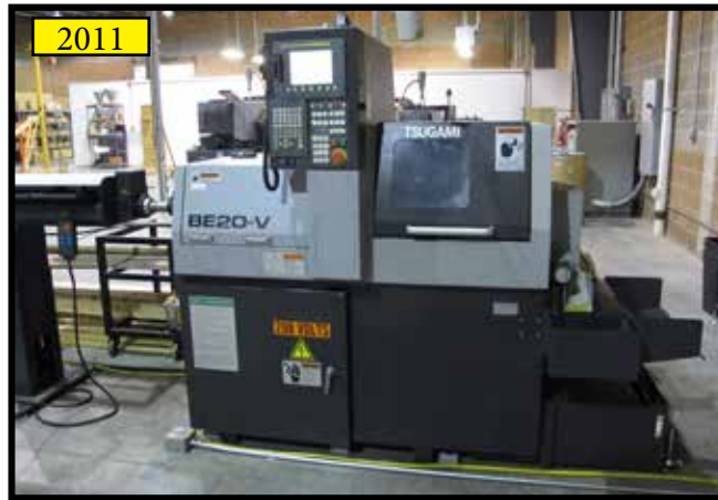
2011 TSUGAMI BE20-V, 5 AXIS CNC SCREW MACHINE, 12,000 RPM, 20 mm CAP, W/LNS BARFEED, FANUC 31i- MODEL A CONTROL SIN: 6015
