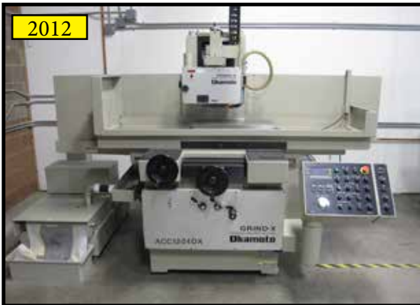
2012 OKAMOTO GRIND X ACC 12-24 DX, 12X24 HYD PROGRAMMABLE SURFACE GRINDER.
