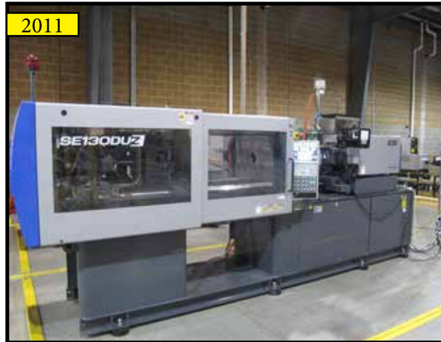
2011 SUMITOMO SE130DUZ, 143 TON DIRECT DRIVE ELECTRIC INJECTION MOLDING MACHINE, 2.9 OZ SHOT, 28.35" X 26.38" PLATTEN SIZE.
