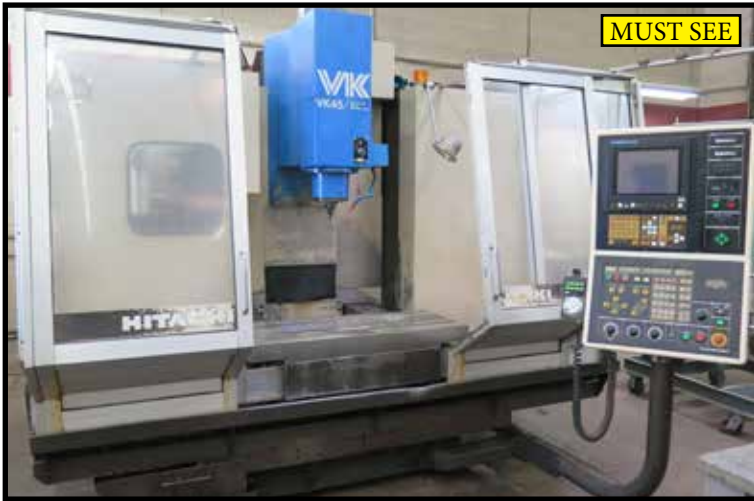
Hitachi Seiki VKK-45 Sliding Column CNC Vertical Machining Center s/n VK-46343 w/ Hitachi Seiki Seicos Controls
