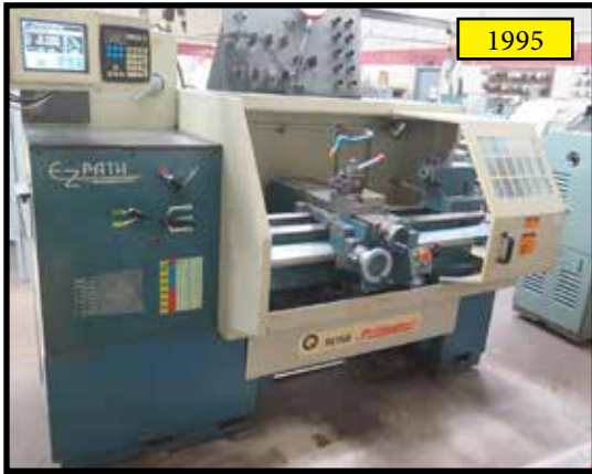
1995 Romi-Bridgeport EZ-Path 17" x 44" CNC Lathe s/n 002-079481- 325 w/ EZ-Path CNC Controls
