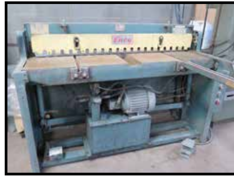
Enco mdl. 130-5345 52" Power Shear s/n 7910008
