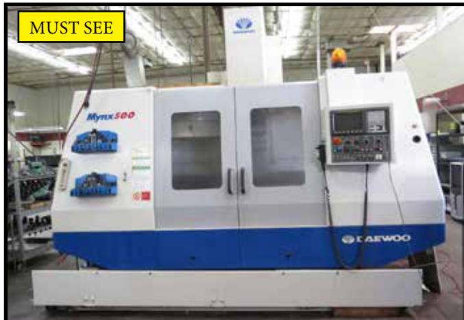
Daewoo Mynx 500 CNC Vertical Machining Center w/ Fanuc Series 21-M Controls, 24-Station ATC, CAT-40 Taper Spindle, 19 1/2" x 47 1/4" Table, Coolant.
