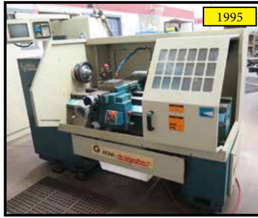
1995 Romi-Bridgeport EZ-Path 17" x 44" CNC Lathe s/n 002-078888-325 w/ EZ-Path CNC Controls
