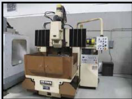
URAWA UB-75 CNC BRIDGE MILL, FANUC 6M CONTROL, 18 ATC, BT-40, 4TH AXIS READY
