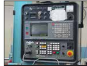
2012 TOSHIBA BP-150.R22 CNC HORIZONTAL BORING MILL S/N 421541 W/ TOSNUC 999 CONTROLS, 60-STATION ATC, CAT-50 TAPER SPINDLE, 6" SPINDLE, 70.9" X 86.6" TABLE INDEXABLE @ 90 DEGREES, 7717 ON HOURS, 2066 SPINDLE HOURS, 1565 CUTTING HOURS.
