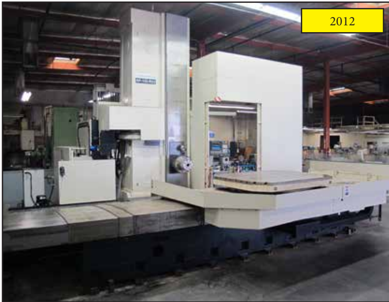
2012 TOSHIBA BP-150.R22 CNC HORIZONTAL BORING MILL S/N 421541 W/ TOSNUC 999 CONTROLS, 60-STATION ATC, CAT-50 TAPER SPINDLE, 6" SPINDLE, 70.9" X 86.6" TABLE INDEXABLE @ 90 DEGREES, 7717 ON HOURS, 2066 SPINDLE HOURS, 1565 CUTTING HOURS.
