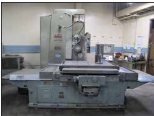
DeVlieg Spiramatic 65K-144 4-Axis CNC Horizontal Boring Mill s/n 4935 w/ Fanuc Series 16-M Controls,
