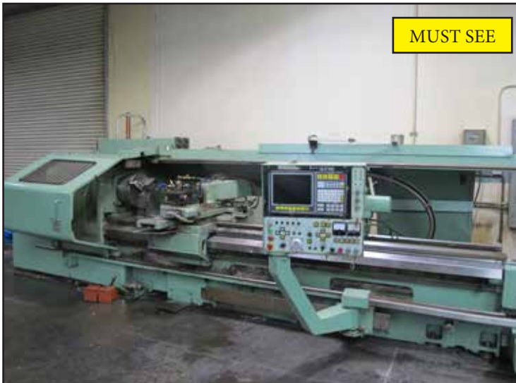
OKUMA LH35-N CNC LATHE S/N S/N 58.1-1867 W/ OKUMA OSP5000L CONTROLS, 6-STATION TURNING TURRET, 4-POSITION TURNING/BORING HEAD, TAILSTOCK, 15" 3-JAW CHUCK, COOLANT.
