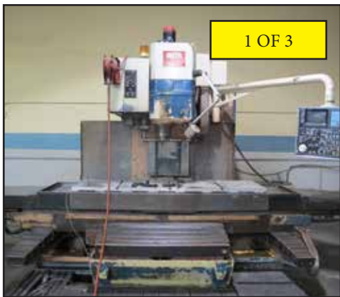
OOYA RE-1MVL CNC VERTICAL MACHINING CENTER S/N VL2110022 W/ FANUC 11M CONTROLS, 36-STATION ATC, CAT-45 TAPER SPINDLE,
