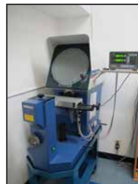
Mitutoyo PH-A14 14" Optical Comparator s/n 009481301 w/ Mitutoyo KA Counter Programmable DRO, Surface and Profile Illumination, 6" x 16" Table.
