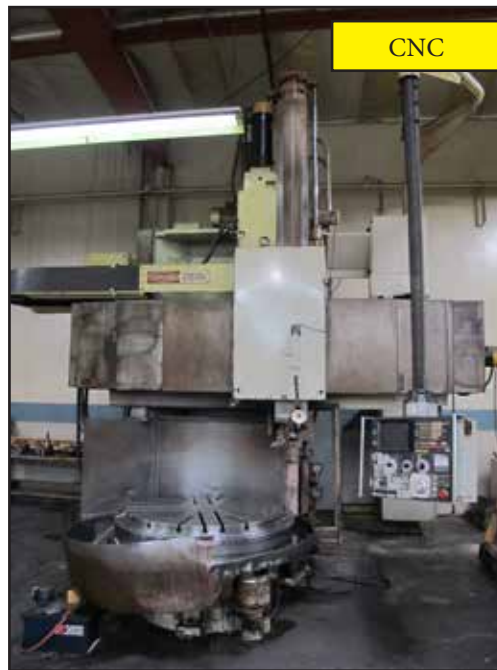
Shibaura TSN-13A CNC Vertical Boring Mill s/n 410107 w/ Fanuc System 6T Controls, 49" Chuck, 67" Max Swing.
