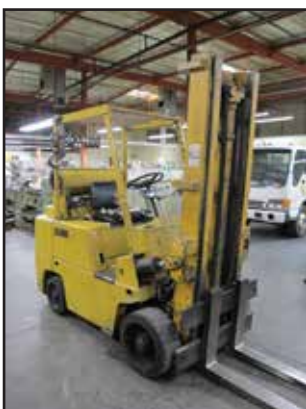
Clark C500S80 8000 Lb Cap LPG Forklift s/n 68524241679 w/ 2-Stage Mast, 171" Lift Height, Solid Tires.
