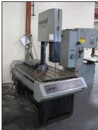
MARVEL SERIES 8 MARK II 18" VERTICAL MITER BAND SAW W/ MANUAL CLAMPING, 45 DEGREE MITER CAPAB.
