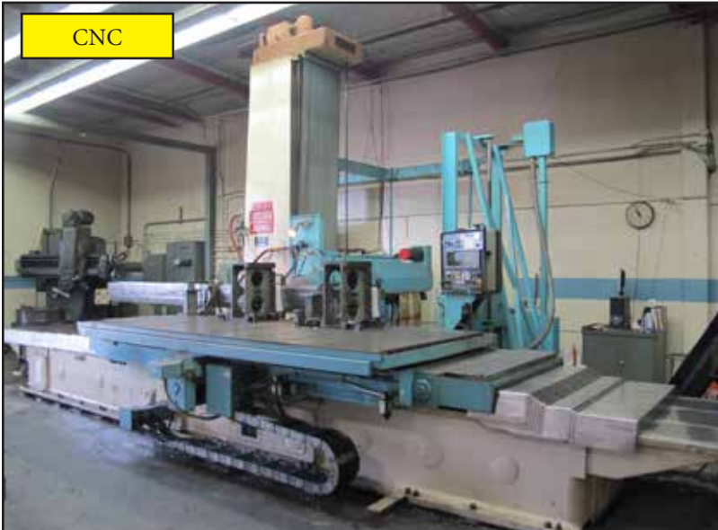
DEVLIEG SPIRAMATIC 65K-144 4-AXIS CNC HORIZONTAL BORING MILL S/N 4935 W/ FANUC SERIES 16-M CONTROLS, HAND WHEEL, 10-1800 RPM, 6" SPINDLE, 50-TAPER SPINDLE, 60" X 144" TABLE, 50" X 72" 4 TH AXIS ROTARY TABLE.
