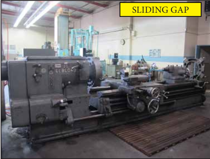
LEBLOND 25" SLIDING-GAP GAP BED LATHE S/N N11244 W/ 200" SLIDE EXPANSION, 5-600 RPM, TAPER ATTACHMENT, INCH THREADING, TAILSTOCK, STEADY REST, KDK TOOL POST, 24" 4-JAW CHUCK.
