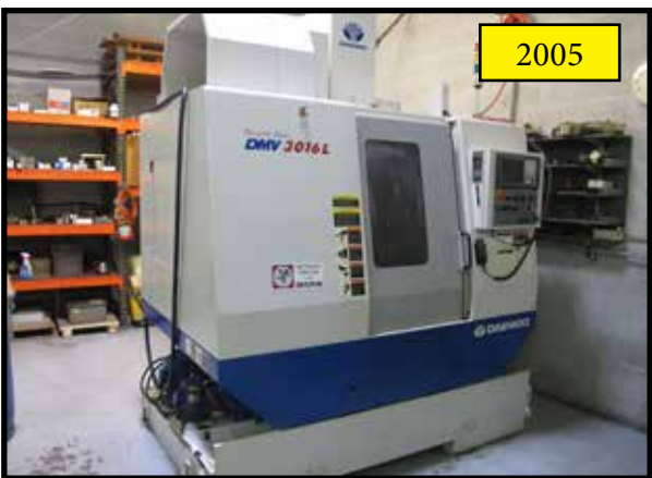
2005 DAEWOO DMV-3016L CNC VMC, DIAMOND SERIES, 8000 RPM, SIDE MOUNT 24 ATC, WITH FANUC I SERIES CONTROL, LINEAR WAYS, 30" X 16.1" X 20.1" (XYZ) S/N NM4100055.
