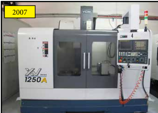
2007 YCM XV SERIES 1250A CNC VMC, W/ FANUC MXP-100i, BT-40 AND W/ CT-40 ADAPTER, LINEAR WAYS, 10,000 RPM, 40" X 20" X 20" (XYZ), S/N 18.
