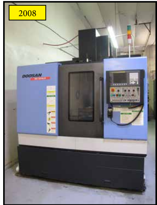
2008 DOOSAN MV-3016LD CNC VMC, W/ FANUC I SERIES CONTROL, 20 ATC, CT-40, LINEAR WAYS, 8000 RPM, 30" X 16 X 20" (XYZ), S/N NM101190.
