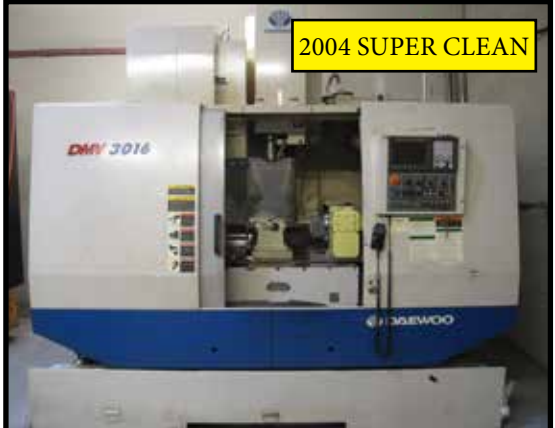
2004 DAEWOO DMV-3016 CNC VMC WITH 4TH AXIS READY, BOX WAYS, SIDE MOUNT 24 ATC CT-40, 30" X 16" X 20" (XYZ), S/N AV1E0260.
