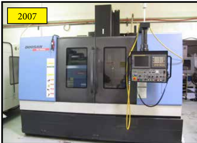
2007 DOOSAN MV-4020D CNC VMC, W/ FANUC 21i-Mb CONTROL, 24 ATC, CT-40, 8000 RPM, BOX WAYS, 40" X 20" X 24.6" (XYZ), S/N AV5E3125.
