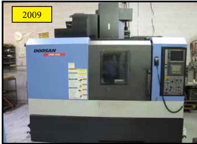
2009 DOOSAN DNM-400 CNC VMC, W/ FANUC i SERIES CONTROL, SIDE MOUNT 20 ATC, CT-40 HOLDER, LINEAR WAYS, 8000 RPM, 30" X 17.1" X 20.1" (XYZ), S/N 4000084.
