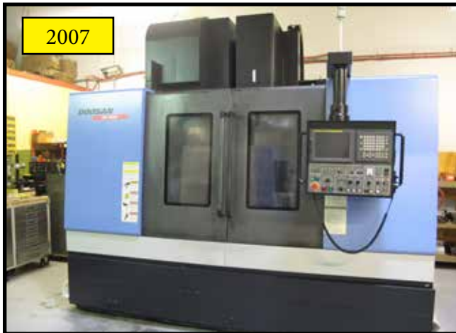
2007 DOOSAN MV-4020 W/ FANUC 21i-MB CONTROL, 24 ATC, COOLANT THRU SPINDLE, SIDE MOUNT 30 ATC, CT-40, 8000 RPM, CERAMIC BEARINGS, KAUKAN OIL CHILLER, BOX WAYS, 40" X 20" X 24.6" (XYZ), S/N AV5E3154. (2007)
