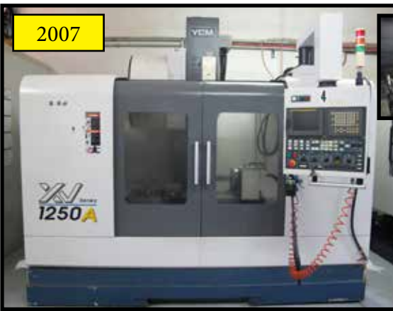
2007 YCM XV SERIES 1250A CNC VMC, W/ FANUC MXP-100i, BT-40 AND W/ CT-40 ADAPTER, LINEAR WAYS, 10,000 RPM, 40" X 20" X 20" (XYZ), S/N 18.
