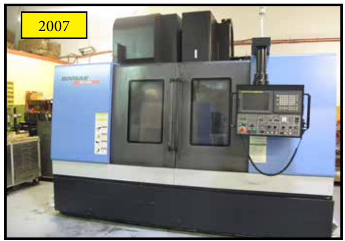
2007 DOOSAN MV-4020 W/ FANUC 21i-MB CONTROL, 24 ATC, COOLANT THRU SPINDLE, SIDE MOUNT 30 ATC, CT-40, 8000 RPM, CERAMIC BEARINGS, KAUKAN OIL CHILLER, BOX WAYS, 40" X 20" X 24.6" (XYZ), S/N AV5E3154.
