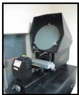
MASTER VIEW 14" OPTICAL COMPARATOR WITH SURFACE LUMINATION.
