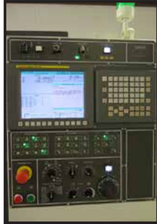
2014 Yama Seiki GS-4000L CNC Turning Center s/n 97F057 w/ Fanuc Series 0i-TD Controls, 12-Station Turret, Hydraulic Tailstock, 2000 RPM, 4.5" Diameter Thru Spindle Bore, 37" Swing Over Bed, 24.4" Max Turning Diameter, 32.7" Max Turning Length, 18" 3-Jaw Power Chuck, Chip Conveyor, Coolant, 331 Metered Hours.
