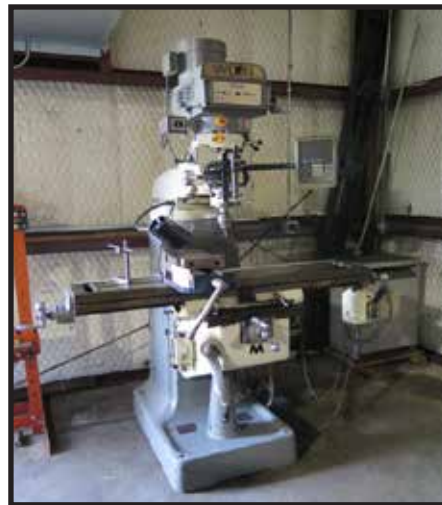
Wilton VS-203 Vertical Mill s/n 4120047 w/ Newall C80 DRO, Mitutoyo Digital "Z" Scale, 60-4200 Dial Change RPM, Chrome Ways, Power Feed, 9" x 49" Table
