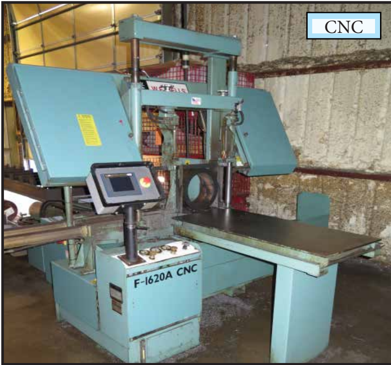
W.F. Wells mdl. F-1620-A 16" CNC Horizontal Band Saw s/n Interface Controls, Hydraulic Clamping and Feeds, Coolant, Conveyor
