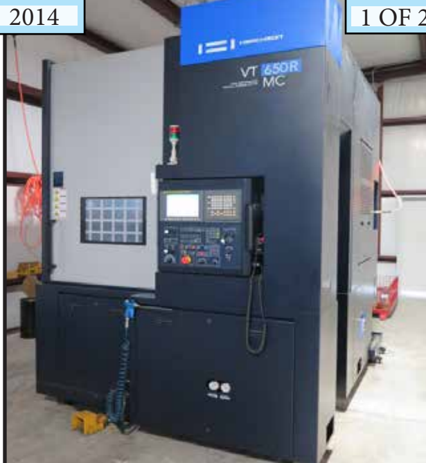
2014 HwaCheon VT-650 R MC CNC Live Turret High Performance Vertical Turning Center s/nM905362H4G A w/ Fanuc Series 0i-TD Controls, Tool Presetter, 12-Station Live Turret, 2000 RPM Spindle, Hand Wheel, Simultaneous Controllable 3-Axis Expansion, 0.001 Degrees "C"-Axis Index Angle, Rigid Tapping, 31.4" Max Turning Diameter, 35.37" Swing Over Bed, 29.47" Max Turning Length, 18" 3-Jaw Power Chuck, 3.9" Diameter Thru Spindle, Axial and Radial Live Tooling @ 3000 RPM, Upgraded Chip Conveyor, High Flow Coolant System, 161 Metered Hours
