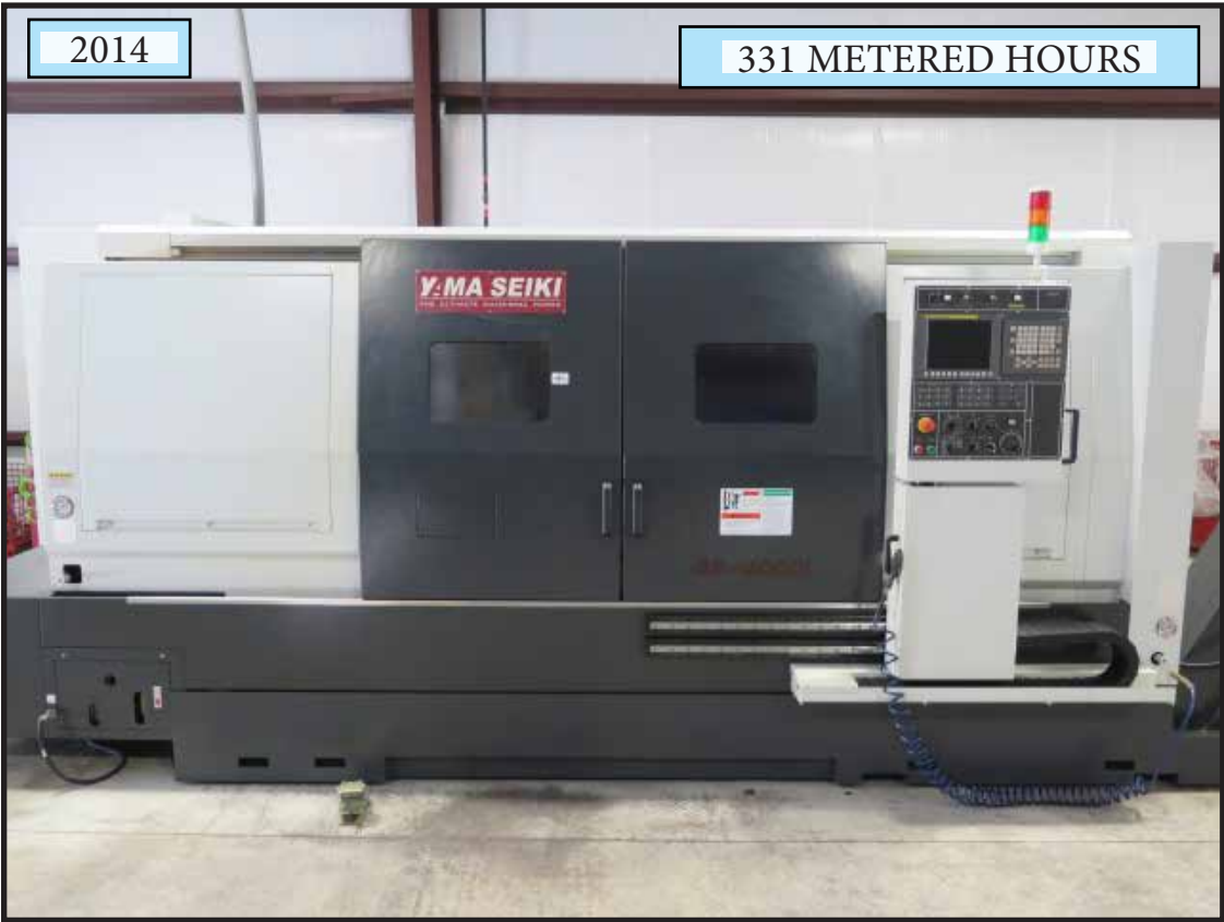
2014 Yama Seiki GS-4000L CNC Turning Center s/n 97F057 w/ Fanuc Series 0i-TD Controls, 12-Station Turret, Hydraulic Tailstock, 2000 RPM, 4.5" Diameter Thru Spindle Bore, 37" Swing Over Bed, 24.4" Max Turning Diameter, 32.7" Max Turning Length, 18" 3-Jaw Power Chuck, Chip Conveyor, Coolant, 331 Metered Hours.
