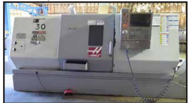
2008 Haas SL-30TB Big Bore CNC Turning Center s/n 3080790 w/ Haas Controls, "A" Package, Tool Presetter, 4" Thru Bore, 12-Station Turret, 2400 RPM, Tailstock, Haas 16DP-50M Gear Box, Haas VOP-B, Rigid Tapping, M19 Spindle Orientation P & R Codes, Intuitive Programming System, Quick Code, USB Port, 15" 3-Jaw Power Chuck, Chip Conveyor, Haas Coolant Filtration System, Coolant
