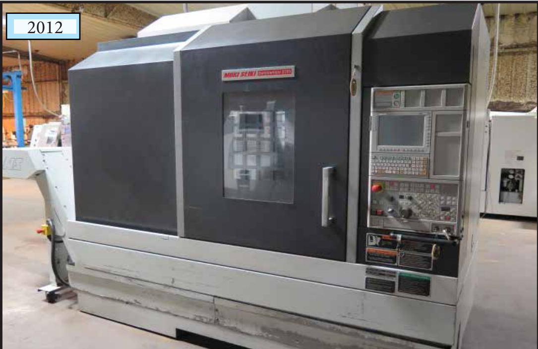
2012 Mori Seiki Dura Vertical 5100 CNC Vertical Machining Center s/n DV005120113 w/ Mori Seiki FOiMD Controls, 30-Station Side Mounted ATC, CAT-40 Taper Spindle, 12,000 RPM Spindle, Thru Spindle Coolant, DDRTI/F, Chip Augers, Chip Conveyor, Chip Blaster High Pressure / High Volume Coolant System, 23 1/2" x 53" Table
