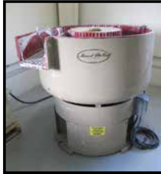
Hammond Roto-Finish Gemini Extended Range Series 48" Media Tumbler
