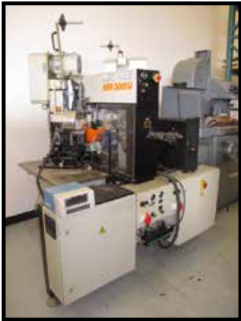
Schaefer Megomat ASM3001U Wire Processing Machine
