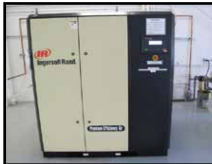
2003 Ingersoll Rand IRN50H-CC 50Hp Rotary Air Compressor w/ Intellisys Digital Controls
