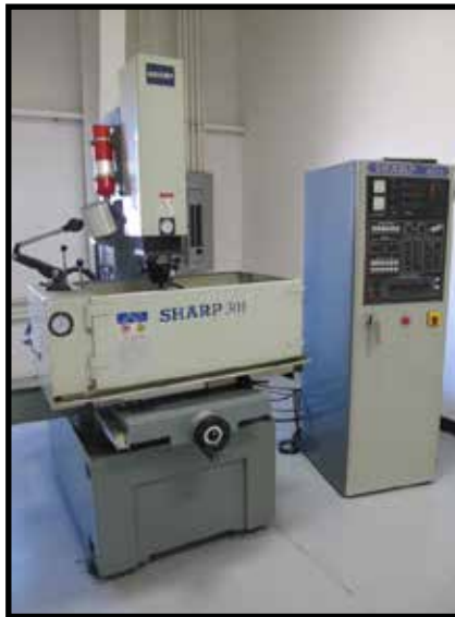
2000 Sharp SED301 Die-Sinker EDM Machine w/ Sharp AZ75 "FUZZY" Control Package, Heidenhain DRO, Fire Suppression, Coolant and Filtration, 423 Metered Hours
