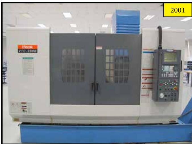
2001 Mazak VTC-200B CNC Vertical Traveling Column Machining Center w/ Mazatrol PC-FUSION-CNC 640M Controls, Renishaw TS27R Tool Measuring System, 24-Station ATC, CAT-40 Taper Spindle, 10,000 RPM Spindle, 3-D High Speed Software Update
