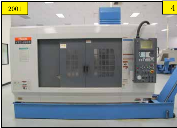
2001 Mazak VTC-200B 4-Axis CNC Vertical Traveling Column Machining Center w/ Mazatrol PC-FUSION-CNC 640M Controls, Renishaw TS27R Tool Measuring System, 24-Station ATC, CAT-40 Taper Spindle, 10,000 RPM Spindle, 3-D High Speed Software Update
