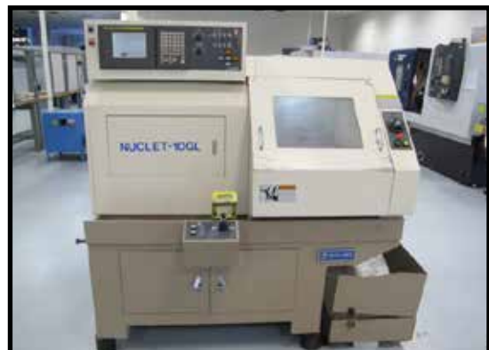
2000 Eguro Nucllet-10GL CNC Gang Tooling Cross Slide Lathe w/ Fanuc Series 21i-T Controls, 5000 RPM Spindle, 5C Collet Closer
