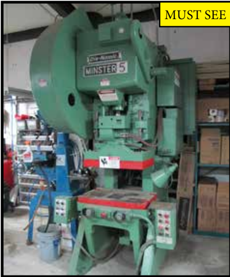
Minster-5 50 Ton OBI Stamping Press w/ 18" x 28" Bolster Area, 14" x 24" Ram Area, Crank Tilting Adjustment
