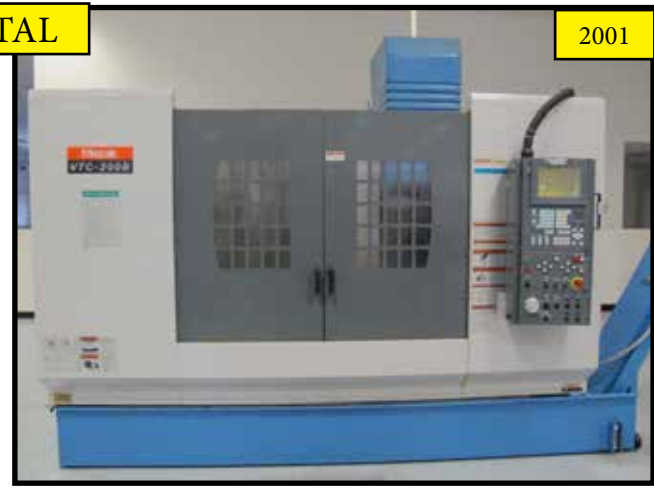
2001 Mazak VTC-200B CNC Vertical Traveling Column Machining Center w/ Mazatrol PC-FUSION-CNC 640M Controls, Renishaw TS27R Tool Measuring System, 24-Station ATC, CAT-40 Taper Spindle, 10,000 RPM Spindle, 3-D High Speed Software Update
