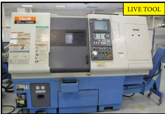
2001 Mazak Super Quick Turn 100MS Twin Spindle Live Turret CNC Turning Center w/ Mazatrol PC-FUSION-CNC 640T Controls, Tool Presetter, 12-Station Live Turret, 6000 RPM Live Tooling, Full "C" Axes on Main and Sub Spindles, 6" 3-Jaw Main Power Chuck, (4) Live Turret Tooling
