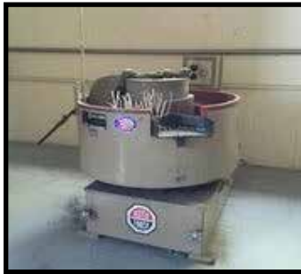
Roto-Finish 21" Media Tumbler s/n ST-1C- 00-A22.
