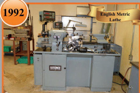
1992 Hardinge Super Precision (ENGLISH METRIC SYSTEM), Acu-Rite III DRO Model HLV-EM, 1.5 HP, S/N HLV-H-13868-T
