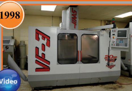
1998 Haas VF-3, Travels 40" x 20" x 25", 2 Speed Gear Box, 7,500 RPM, Auger, 4th Axis Pre Wire S/N 14279
