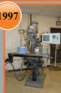
1997 Bridgeport EZ Trak DX CNC Knee Mill, Travels 30" x 12" x 16"
