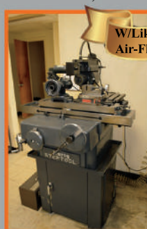
Harig Steptool Grinder Model 2023GWHAR, includes Harig Air-Flo tool box for sharpening and relieving cutters
