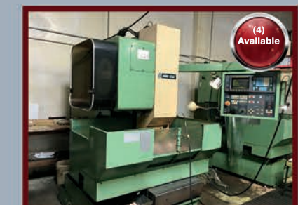
(4) Mori Seiki MV-Junior CNC VMC, Fanuc MF-M4 Control, 20 ATC, 4th Axis Ready
