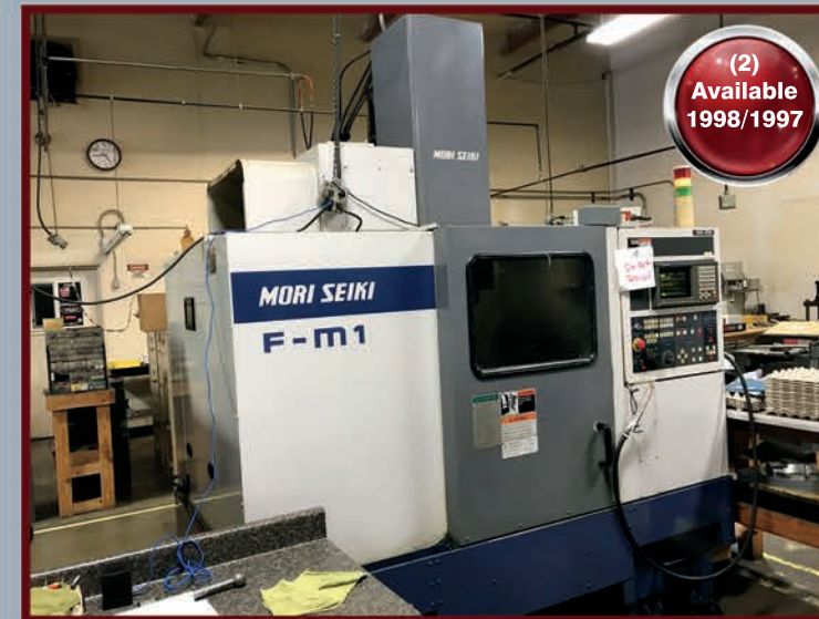
(2) 1998/1997 Mori Seiki F-M1 CNC VMC, Fanuc MSC-521 Control, 20 ATC
