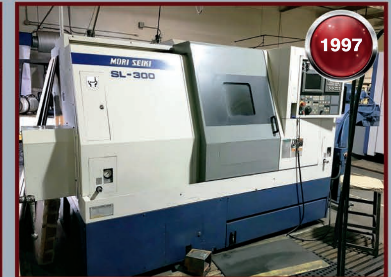
1997 Mori Seiki SL-300A CNC Lathe, Fanuc MSC-518 Cntrl, 12" Kitagawa 3-Jaw Ck, 12 Station Turret, Tailstock, Chip Conveyor
