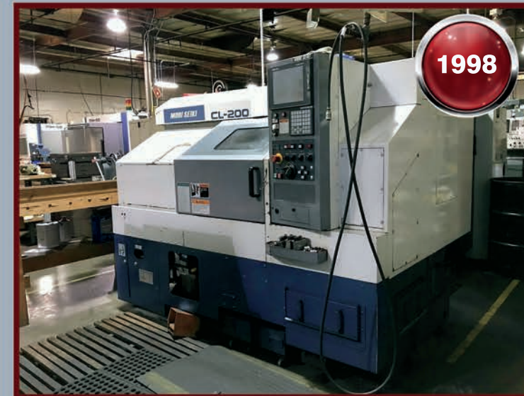
1998 Mori Seiki CL-200B500 CNC Lathe, MSC-803 Control, 8" MMK 3-Jaw Chuck, 10 Station Turret, Tailstock
