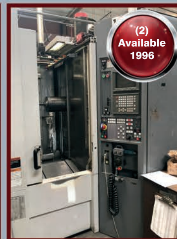
(2) 1996 Mori Seiki SH-50's, 19.7"/19.7" Pallets, 24.8" x 23.6" x 25.6" Travels, 12,000 RPM, Cat 40 Taper
