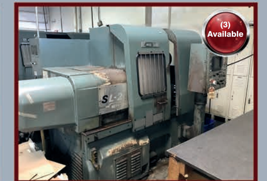
(3) Mori Seiki SL-2H CNC Lathe, Fancu 11T Control, 10" Kitagawa 3-Jaw Chuck, 12 Station Turret
