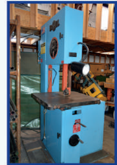
2001 DoAll 2013-V Vertical Band Saw, Band Length 154"
