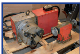
Haas HRT-210 Brushless 4th Axis Rotary Table with Tailstock
