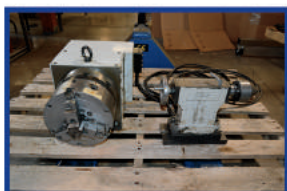
Haas HRT-210 Brush Type 4th Axis Rotary Table with Tailstock
