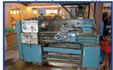
Enco Engine Lathe 111-1445 Platinum Plus DRO Control
