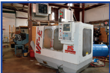
1997 Haas VF-E, 4th Axis wired, Rigid Tap, P-Cool, Floppy, Chip Auger
