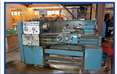
Enco Engine Lathe 111-1445 10" 3 Jaw Chuck, Tailstock, Enco Platinum Plus DRO Control
