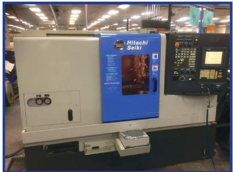
2001 Hitachi Seiki HT20SII turning center s/n NR30701 w/LNS barfeed system, misc collets, 8" hydraulic chuck, 2" Bar capacity, Parts catcher, Tailstock, 5,000 rpm, 17" Swing, 12 Position Turret, Chip Conveyor, Seicos Control
