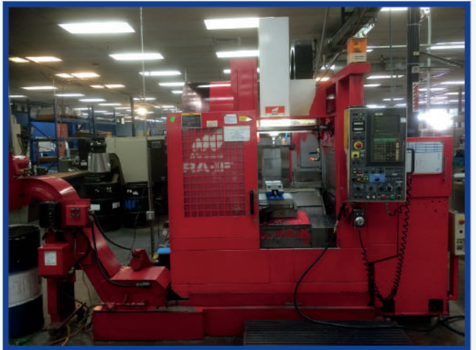
1996 Matsuura RA-1F Vertical Machining Center, pallet changer, s/n 951011601, 2 Pallet Changer, 15,000 RPM, 21" X 15" X 18" Travels, 40 taper, 30 Position Tool Changer, Chip Conveyor
