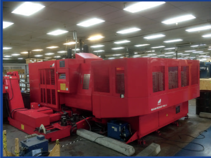
1998 Matsuura MAM-500H-11PC Horizontal Machining Center-11 pallet system, s/n 980613196, Matsuura System i80 Control, Includes 11 tombstones and approx. 70 BT40 Taper tool holders, 4th Axis, 19.6" X 18.5" X 17.72" Travels, 12,000 RPM, 120 Position Tool Changer, Chip Conveyor
