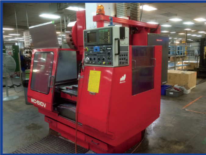
1991 Matsuura MC-510V 3-axis vertical machining center s/n 910609401 with 15" x 30" Table, 20" X 14" X 18" Travels, 5/7HP, 60-6,000 RPM, 20 Position ATC, 40 Taper, Yasnac MX3 Control
