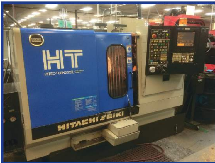
1995 Hitachi Seiki HT20SII turning center s/n NR24813 w/LNS barfeed system, misc collets, 8" hydraulic chuck, 2" Bar capacity, Parts catcher, 5,000 rpm, 17" Swing, 12 Position Turret, Chip Conveyor, Seicos Control
