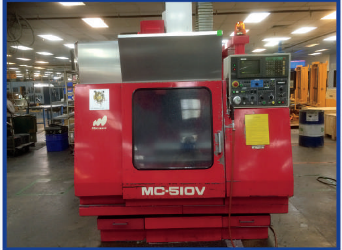
1991 Matsuura MC-510V 3-axis vertical machining center s/n 910709471 with 15" x 30" Table, 20" X 14" X 18" Travels, 5/7HP, 60-6,000 RPM, 20 Position ATC, 40 Taper, Yasnac MX3 Control
