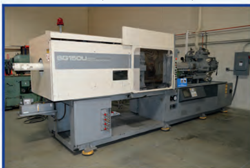
1994 Sumitomo 150 ton IMM, Model SG150U.S-M IV, SN MOHT8694, HKO, Plummed for Air Blast, RI
