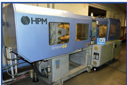
1997 HPM Universal 60 ton, Model T60-230, Barber-Colman Control, HKO
