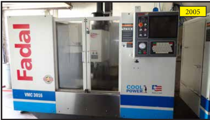
2005 Fadal VMC3016HT CNC Vertical Machining Center s/n 032005027397 w/ Fadal Multi Processor CNC Controls, 21-Station ATC, CAT-40 Taper Spindle, 10,000 RPM, High Torque Spindle Motor, AC Drives, 4 meg Memory Expansion, High Speed CPU, Rigid Tapping, Graphics
