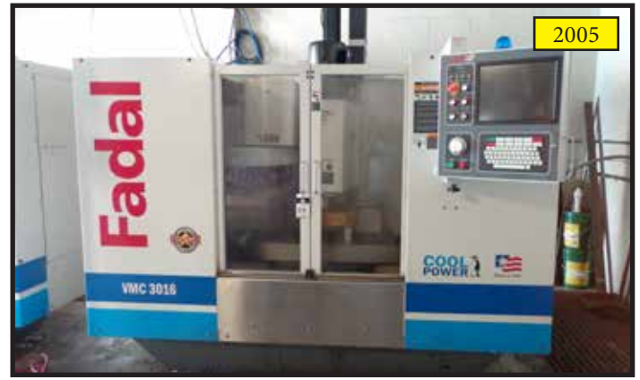
2005 Fadal VMC3016HT CNC Vertical Machining Center s/n 032005027396 w/ Fadal Multi Processor CNC Controls, 21-Station ATC, CAT-40 Taper Spindle, 10,000 RPM, High Torque Spindle Motor, AC Drives, 4 meg Memory Expansion, High Speed CPU, Rigid Tapping, Graphics
