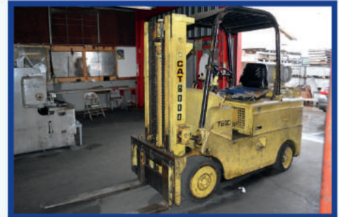
Catipillar Fork Lift, Propane, Includes Battery Charger as seen, Model T80C, 8000lbs Capacity, Standard Mast, 122" Fork height, 24" Load Center, Hours Read 3330.6
