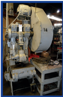
Niagara A3 Punch Press, 45 Ton, 4" Shut Height, 2.25" Adjustment, With Steel Table and All Included Contents
