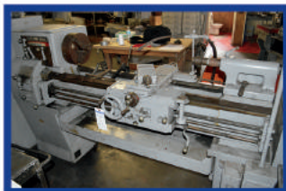
Leblond Regal Lathe with 10" Chuck and 64" Centers
