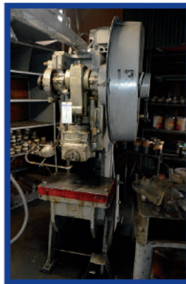
Niagara A35, 35 Ton Press 10.25" Shut Height with 2.25" Adjustment, Steel table with contents Included
