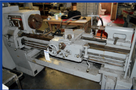
Leblond Regal Lathe with 10" Chuck and 64" Centers
