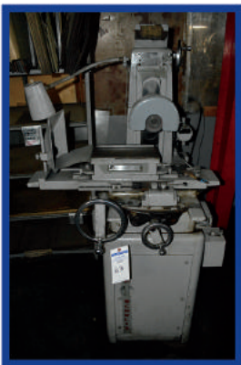
Boyar Schultz Grinder, 12x6 Capacity, With Magnalock Corp Model HR612C Chuck
