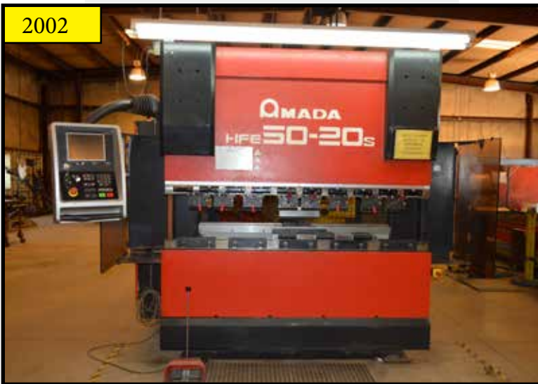
2004 AMADA HFE 50-20S, 6FT X 50 TON CNC HYD PRESS BRAKE, 7 AXIS CONTORL, S/N V040157.
