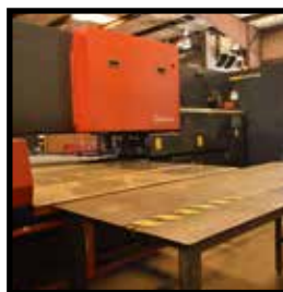
2000 AMADA APELIO 367V III, CNC LASER PUNCH MACHINE WITH 2000 WATT LASER, 33 TON PUNCH SYSTEM, 58 STATION TURRET, AUTO INDEX, WITH AMADA MST1530 LOADING SYSTEM, S/N 33670050.
