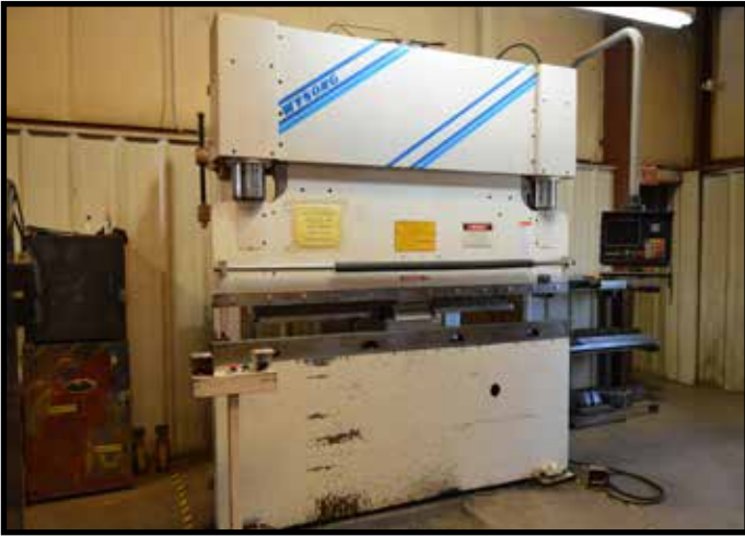
WYSONG MTH-100-96, 8FT X 100 TON CNC HYDRAULIC PRESS BRAKE WITH AUTOBEND 7 BACK GAGE, S/N MT15-113.
